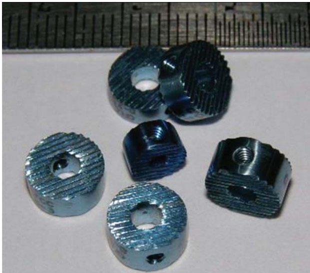
Fig. 1. Photograph showing the various sizes of the spacers. The flat surface has serrations to make the surface rough. The hole with serrations on the side of the implant is meant for the spacer holder. The hole in the center of the flat surface is meant to assist in arthrodesis.
