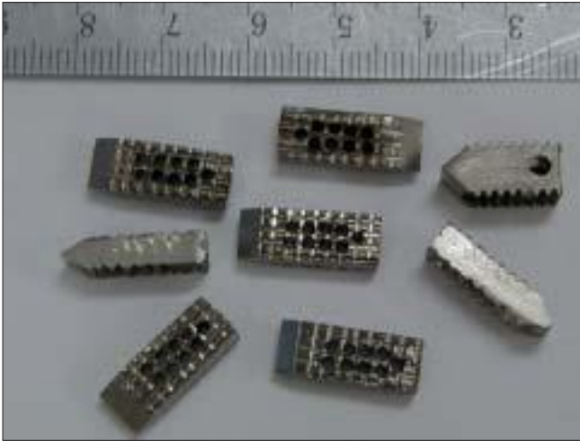
Figure 4: Picture showing the spacers of various sizes. The spacers are made of titanium and have spikes. There are multiple holes within the body of the spacers for assistance with bone healing. The spacers are tapered at leading edge to assist insertion within the joint. The base of the spacer has a transverse slot for stability of a suitable osteotome during hammer insertion
